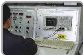
Impulse voltage test (600kV)
