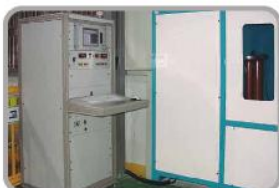
Partial discharge test (100pf)
